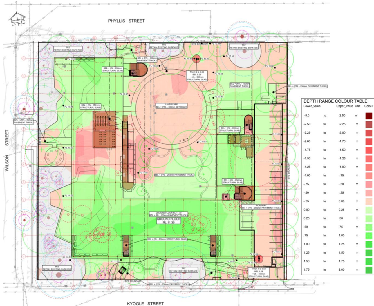
Figure 11: Earthworks cut and fill volumes plan (Source: TTW)
